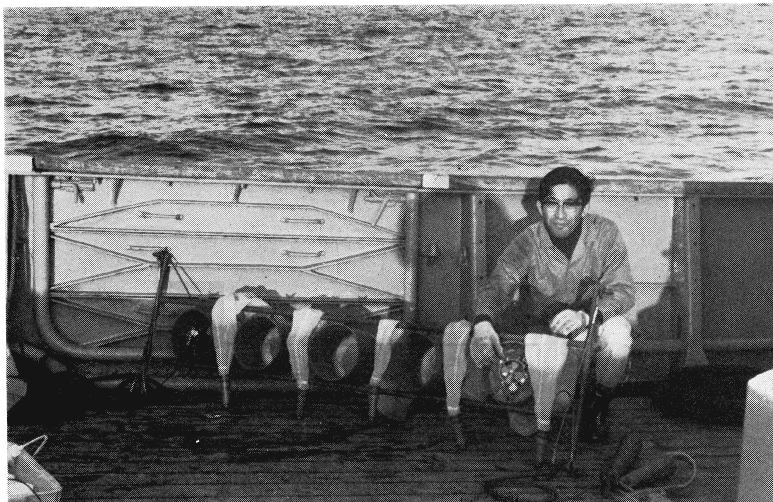
Fig. 2. An assembly of the Multilayer Surface Zooplankton Sampler on board the R/V Mizuho Maru.
