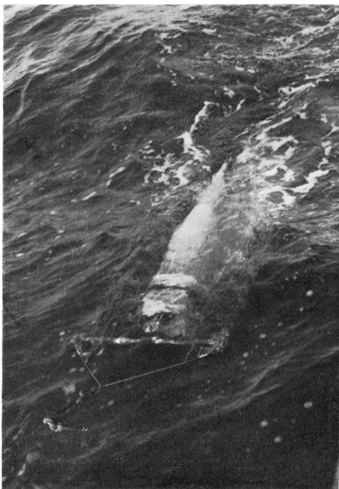
Fig. 4. The Multilayer Surface Zooplankton Sampler swimming in the Sado waters (being towed by R/V Mizuho Maru).
